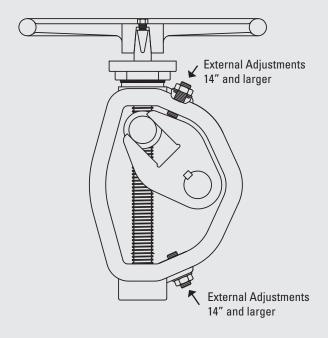
450 FT-LBS. OVERLOAD PROTECTION. Overloads developed by excessive input torque are absorbed instead of being transmitted to mechanism and valve. Lets you apply up to 450 ft-lbs. input torque at open and closed positions without damage to valve or operator.
