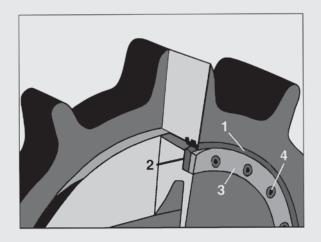
**RUBBER TO STAINLESS SEATING** provides bubble-tight, permanent closure.
