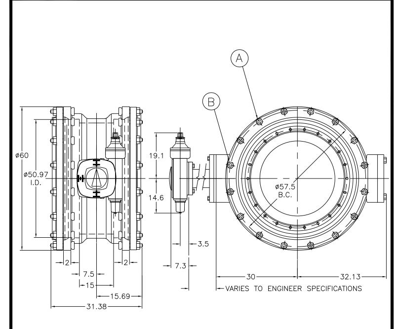
NOTE 2: VALVE SHAFT WILL MEET OR EXCEED REQUIREMENTS OF SHAFT TABLE PER AWWA STANDARD C-504 FOR APPLICABLE CLASS.
