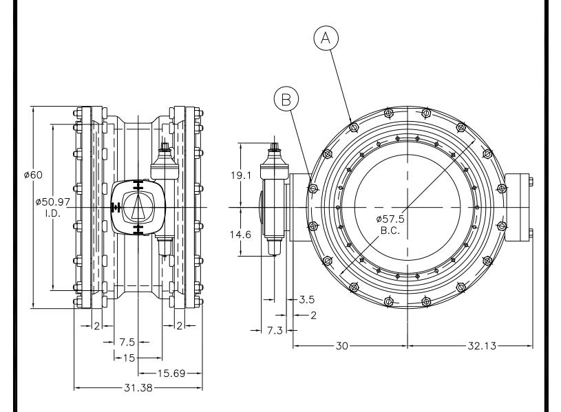
NOTE 2: VALVE SHAFT WILL MEET OR EXCEED REQUIREMENTS OF SHAFT TABLE PER AWWA STANDARD C-504 FOR APPLICABLE CLASS.
